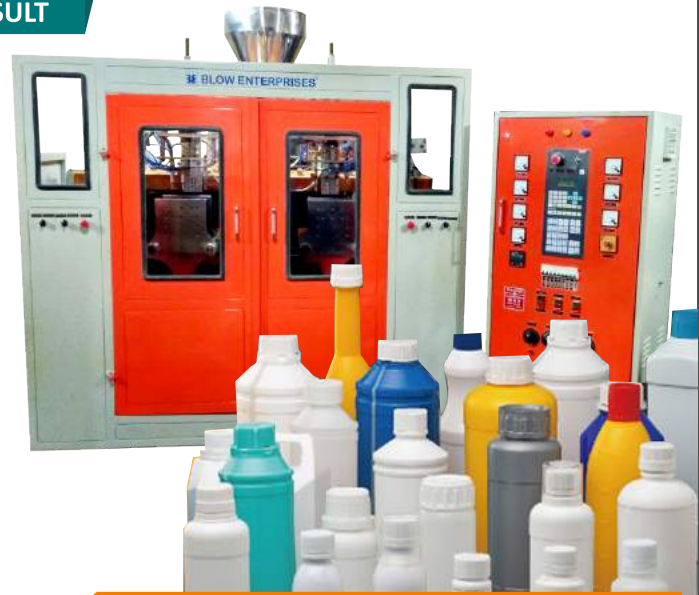
2 Ltrs. Double Station / 4 Cavity Rotary Auto Deflashing
